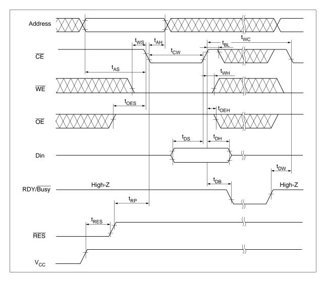
Byte Write Timing Waveform (2) (CE Controlled)
